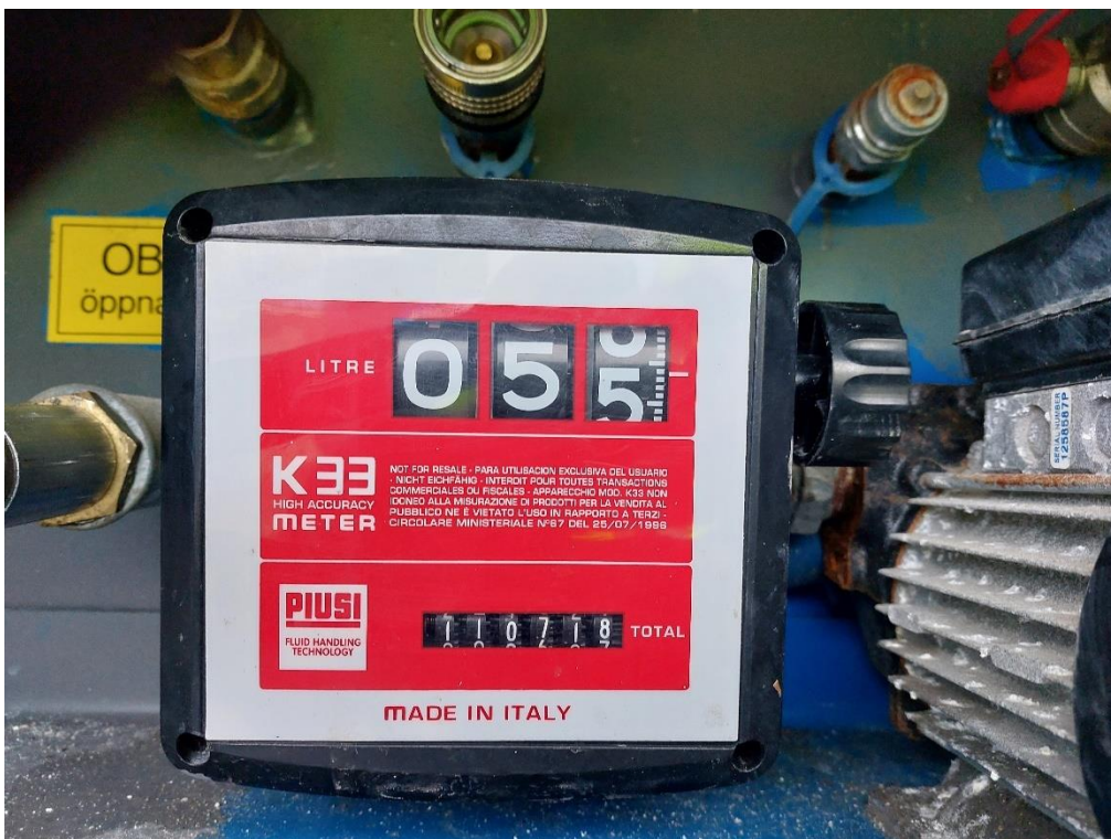
Figure 23. Reading on fuel meter after day 3, week 2. Eco mode + Seismic; 55,4 liters.
