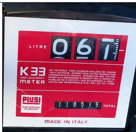
Figure 2. Meter not reset in the morning of 15 Feb., 55.5 l from Thu 10/2 + 6.2 liters from the morning of 15 Feb. after the weekend transport and repair gives 61.7 liters. Compare total fuel used from Thursday 10 Feb. to Tuesday 15 Feb., 3003 to 3006 liters. Only 3 liters. Total volume here is about 110517 liters.
