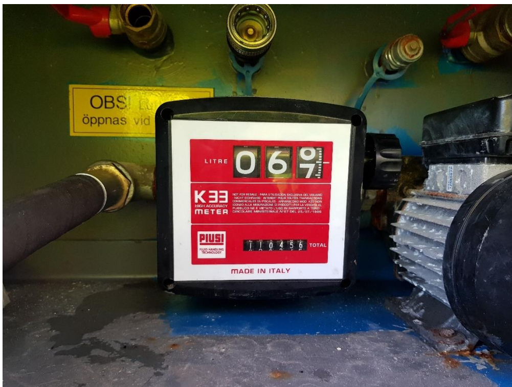
Figure 11. Reading on fuel meter after day 2, week 1. Eco mode; 67,5 liters.
