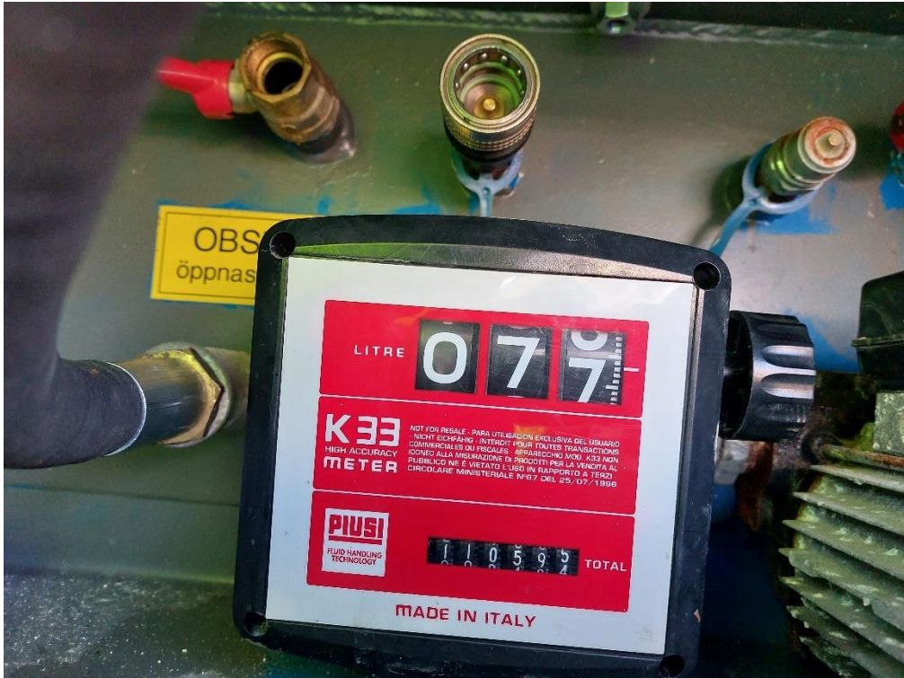
Figure 18. Reading on fuel meter after day 1, week 2. Standard mode with high frequency; 77,3 liters. (Three liters are to little?)
