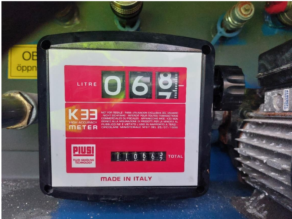
Figure 20. Reading on fuel meter after day 2, week 2. Eco mode; 67,7 liters.
