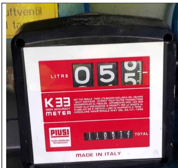
Figur 2. Refueled volumen in the evening 10 Feb., 55.5 liters. The total reading is approximately 110511 liters.
